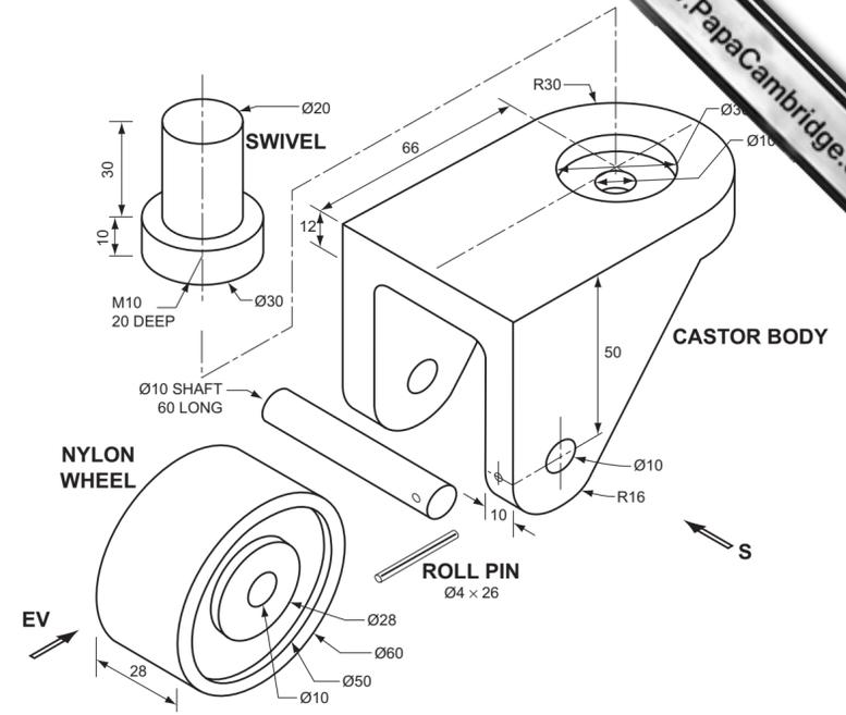
DRAW THE SYMBOL FOR THE ANGLE OF PROJECTION USED HERE
